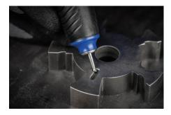
**Note:** Extended shank burs are not suitable for robotic or stationary applications. Risk of bending. Use only rigid clamping systems/power tools. Extended shank burs can be shortened if required.
